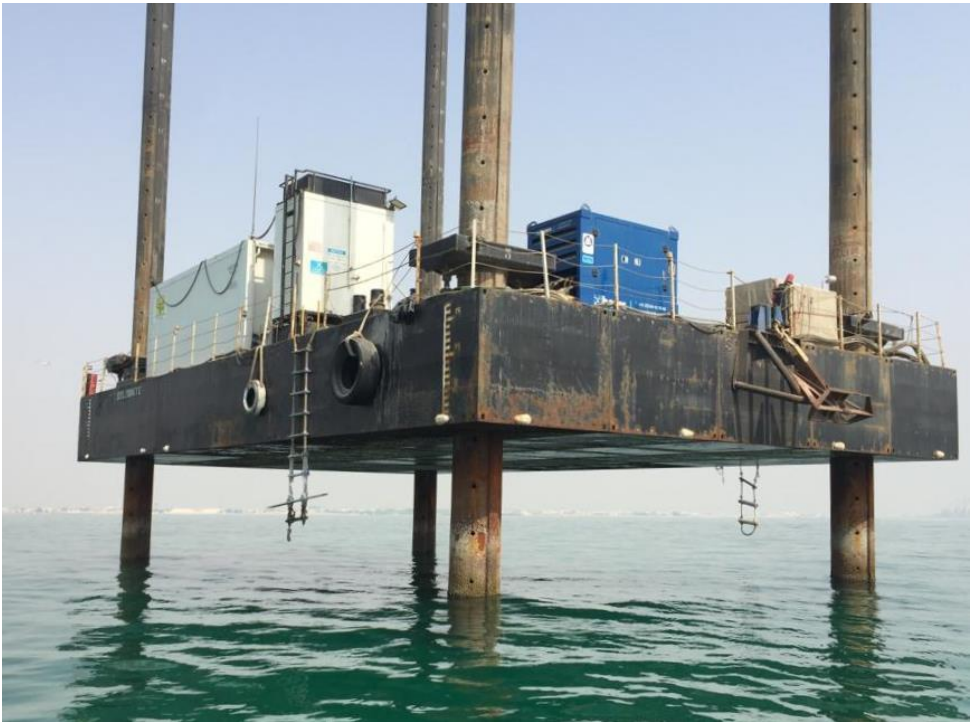
Plate 2. JUB type for installation of WTG in offshore environments
