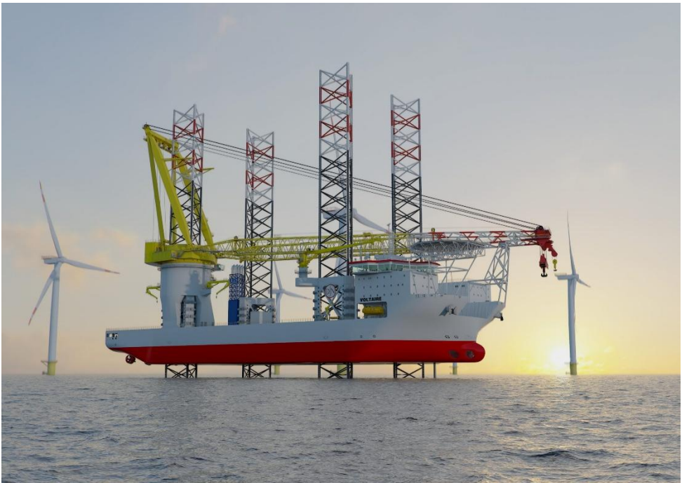
Plate 2. JUB type for installation of WTG in offshore environments
